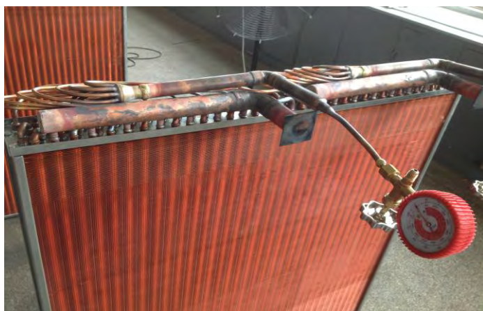
Manufacturing of Evaporator Coil with Copper Fins
