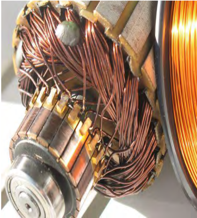
Motor damage winding
