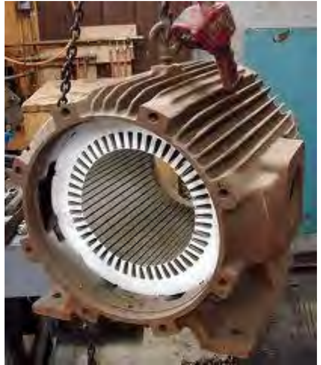
Damage Winding Removed
