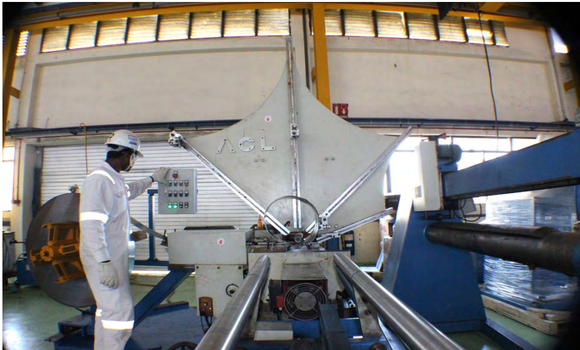
Spiral Ducting Fabrication Machine
