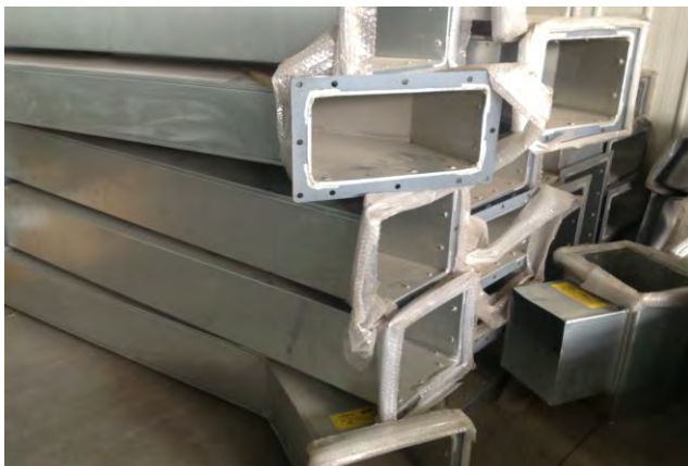
G.I Rectangular Ducting
