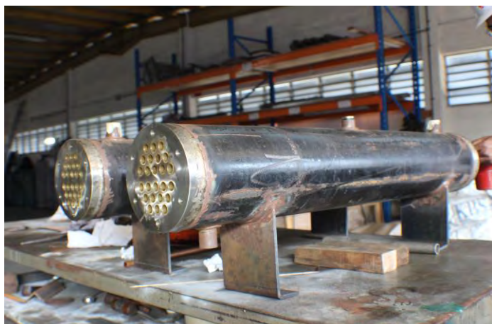
Fabrication of New Condenser
